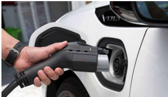
Step 1: Plug in the charging interface
